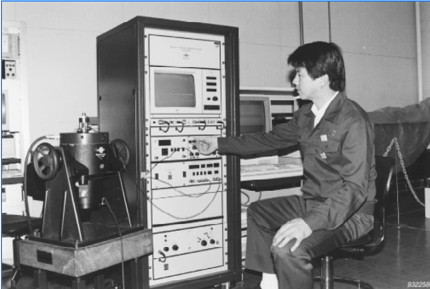
Fig.5 Vibration Transducer Calibration System Type 9610 in use at the Calibration Center
